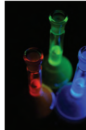
Polar OLED materials showing photoluminescence under a 50Hz, 365nm UV light
